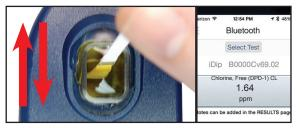
Tap '**SELECT** Test' at the top. Tap Chorine, Combined (DPD-3) CL. The iDip and app will both display Combined Chlorine.
